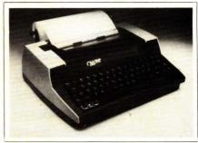
The Z80-μP-based Model MSR 744-8B terminal includes a 62-key keyboard that generates 128 ASCII characters. The battery-backed-up memory can store 8k characters. The printer includes a 256-character buffer and furnishes 30-cps performance. Fourteen character densities range from 5 to 20 cpi; a graphics mode provides 120-dot/in. horizontal, 60-dot/in. vertical resolution.
