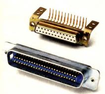
Low-cost filtered input/output connectors. Our new cost-effective design uses stress-isolated NPO dielectric filter chips to eliminate conducted interference in each line. Available in a full range of D-subminiature and ribbon connector types and sizes, the connectors are intermateable with most existing industry standard non-filtered products. A pricing break-through, these filtered connectors can be matched to your insertion loss and band-pass requirements by capacitance value selection.
