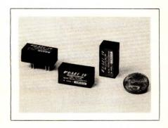
DIP-SIZED CONVERTERS. The CA Series of dc/dc converters provides unregulated, isolated single and dual outputs. Maximum output power is 1.5W and the units withstand 1000V dc at 100-M $\Omega$  input-to-output isolation. The converters come in 16-pin DIP-compatible packages. Power foldback furnishes indefinite short-circuit protection. The units have only eight leads in a staggered pattern that ensures proper orientation. The missing leads also allow extra room under
