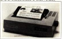
Model H80 prints 27 cps in a near-letter-quality mode and 140 cps in a draft-quality mode. Able to produce pica and elite characters, the dot-matrix printer features overstrike, proportional-character and condensed- and expanded-print capability. It can produce half-size and superscripts and subscripts. It accepts fanfold and single-sheet paper from 5 to 10 in. wide and can print an 8-in.-wide line. It also accepts roll paper.
