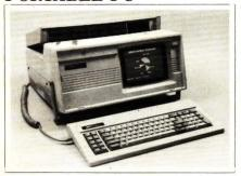
Compatible with the IBM PC, the Z-160 PC features a detached keyboard, four open expansion slots and 128k bytes of dynamic RAM, upgradable to 640k bytes. The unit's single or dual top-loading disk drive accepts 5¼-in. IBM-format double-sided, double-density diskettes.
