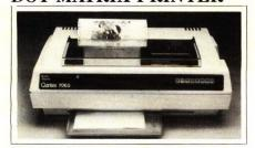
Model 7065 operates at 300 cps in draft mode, 125 cps in near-letter-quality mode, and 65 cps in letter-quality mode. In its graphics mode, it provides resolution of 144×144 dots/in.<sup>2</sup> and repetition rate of 1500 dots/sec per activated needle.
