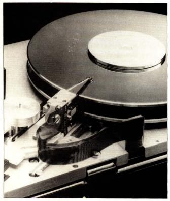
Formatted as 306 cylinders to maintain compatibility with IBM PC/DOS software, Cogito Systems' Model CG912 half-height Winchester uses less than 12W.
