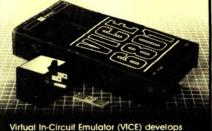
single-chip microcomputer programs for the 6801/68701 and programs on-board EPROM. A cost and time effective way to program the 6801/68701 for \$695.
