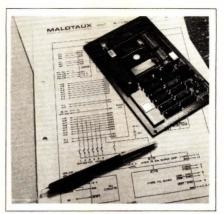
The board contains two 8-bit bidirectional I/O ports, two 16-bit timer/counters and one 8-bit I/O shift register. Other features include a serial RS-232C/V.24 interface, 20 parallel (6522 VIA) I/O lines and the capacity for 32k bytes of EPROM and 8k bytes of RAM. 1950 Dfl. Malotaux Electronic Systems Design, Dorpsstraat 74, 3732 HK, De Bilt, Holland. Phone (030) 770105. TLX 47825.
