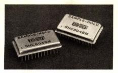
Adding an input-buffer option to a fast industry-standard 12-bit T/H amplifier, this hybrid from Burr-Brown Corp comes in a metal "bathtub" DIP.
