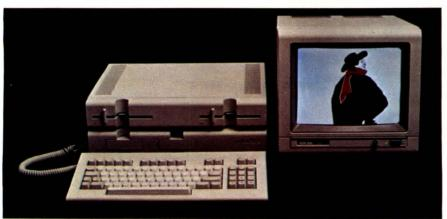
A custom graphics-coprocessor and display-processor chip set are components in the Mindset personal computer, an 80186-based machine that sells for only \$1200 in its basic configuration. The coprocessor performs raster operations that give the Mindset seamless graphics and smooth animation. The Mindset's display, indicative of an industry trend, is completely bit-mapped for both graphics and text.
