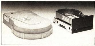
**Two faces of data storage** are Seagate Technology's 100M-byte half-height 8-in. ST8100 Winchester and its 12M-byte 5¼-in. ST412 Winchester.
