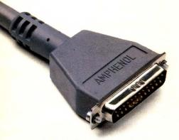
Shielded data communication cable assemblies. For compatibility with systems environments, Amphenol® interface bus cables are multi-shielded designs featuring double-shielded cable with additional shielding around the inner data bus lines. IEEE488-1975 style bus cables are terminated with 24-contact connectors.
