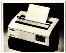
A 24-pin printhead composed of 8-mil-diameter print wires allows Model P1340 to provide 80-column letter-quality output at 54 cps. A draft-quality mode operates at 144 cps (12 cpi) or 120 cps (10 cpi).
