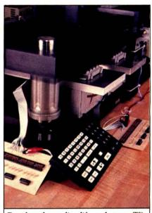
Based on demanding life-cycle tests, TI's durable conductive-rubber keyboard can operate reliably up to 10 million cycles.
