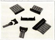
For use with 0.05-in. flat ribbon cable, FT Series insulation-displacement connectors include ejector latches that ensure positive locking of the socket to the header as well as easy detachment. Available with or without strain relief, the headers feature a straight or right-angle design with solder tail. Polarized for correct socket-to-
