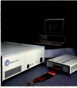
ALL OF THIS...AND GENERIC, TOO Microcosm's emulators are easily upgraded in your lab. Changing from 8086 to 8088 support or from 80186 to 80188 support is as easy as replacing the emulator's target processor and throwing a switch. Upgrading from the 8086/88 emulator to an 80186/188 emulator just means buying an additional probe module. No need to buy the whole package.
