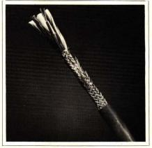
The 8162 Series multipair data cables combine low capacitance (12.5 pF/ft) with a foil and 65%-coverage braid shield and chrome/PVC jacket to allow extended-distance data transmission in RS-232C and RS-422 applications. Shielding on each pair minimizes crosstalk.
