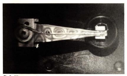
Fig C—When you see fringes across the time-average hologram of the flexure, you've found one of its resonant frequencies.
