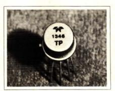
OP AMPS. Combining JFET/bipolar technology and dielectric isolation, Models 1346 and 1347 provide ±250-fA bias current, ±100-μV offset voltage, 2-MHz unity-gain bandwidth and 30-mW power consumption. The amps are suitable for such applications as precision long-term integrators, high-impedance buffers and low-drift track/hold amplifiers. Housed in 8-lead TO-99 packages, the amps
