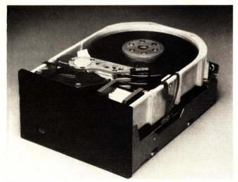
**Using plated media,** *Tandon Corp's Model TM705 stores 50M bytes of data and costs less than \$1000 in large OEM quantities.*
