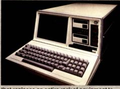
The ADS 100 is a portable unit that replaces an entire rack of equipment to accept data from multiple sources including PCM, PAM, and analog (fm) inputs, as well as time and MIL-STD-1553A/B streams. Its bit-slice processing power can limit check, compress, or convert data at real-time rates. Or preprogram the ADS 100 to solve specific problems of your application. It even provides quick-look capability on the data.
