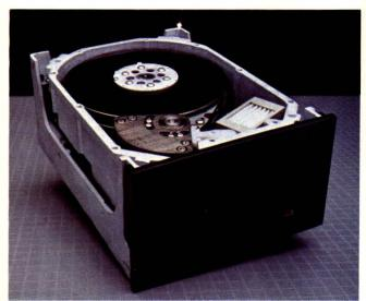
Storing 100M to 200M bytes of data, Micropolis Corp's 1350 Series of 51/4-in. Winchester drives come with an ESDI interface.
