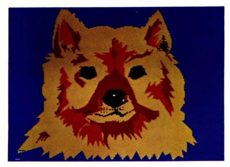
A fully bit-mapped display in NAPLPS (North American Presentation Level Protocol Syntax) format demonstrates the color capability of Texas Instruments' advanced video display processor. Drawing from a 512-color palette, the chip can modify its 16 display colors on every horizontal retrace for subtle shading effects.
