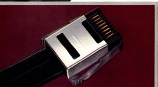
Shielded Data Link connectors available in 4, 8, 16, 24 contact configurations. Insulation-displacing design provides redundant contact on each conductor. Built-in polarization/keying system.
