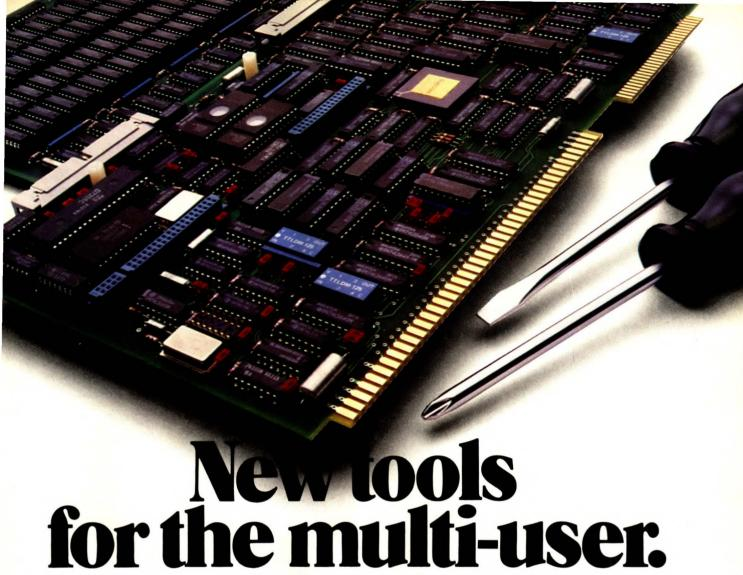
SBE's new 8 Mbyte Multibus 10 MHz 68000 CPU with memory management and no wait states.
