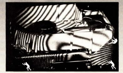
The figures tugging and pulling on this  $5 \frac{1}{4}$  inch disk drive have been sketched in to help visualize the nature of the thermal deformations revealed by the holographic fringe pattern.
